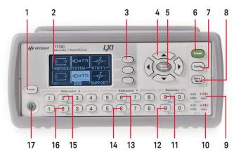
Figure 4. 11713C front panel features
